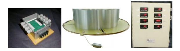
The above left picture shows the rotating Transmitter for the 8 RTD's (cover removed to show connections for the RTD's), the induction power/data coils (during testing in Schenectady) in the center, and the Receiver (digital to analog output device) on the right. The Receiver is equipped with optional panel meters providing y=mx+b unit translation (analog voltage to scaled temperature outputs).
